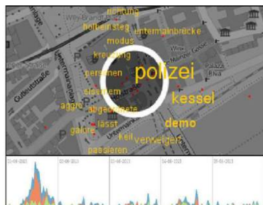
Fig.3. The Content Lens could be used in the third task to assess the ongoing situation in Frankfurt. The three largest tags say police, encircle/em-pocket, and protest. The view below shows the volumes of positive (red) and negative (green) sentiment Tweets for the keyword police in a temporal overview.
