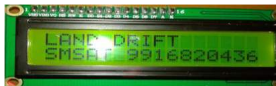
Fig12. Alerting message for landslide
