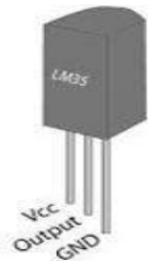
fig 4 pin diagram of temperature sensor
