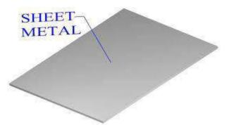
The coils are formed by running a continuous sheet of metal through a roll slitter. The thickness of sheet metal is commonly specified by a traditional, non-linear measure known as its gauge. The larger the gauge number, the thinner the metal. Commonly used steel sheet metal ranges from 30 gauge to about 7 gauge. ISSN (Online) : 2456-5717 21 Gauge differs between ferrous <u>(iron based)</u> metals and nonferrous metals such as aluminum or copper; copper thickness.
