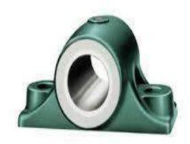
Low-speed pins and bushings are a form of journal bearing in which the shaft or shell generally does not make a full rotation. The partial rotation at low speed, before typically reversing direction, does not allow for the formation of a full fluid film and thus metal-to-metal contact does occur within the bearing. Pins and bushings continually operate in the boundary lubrication regime.
