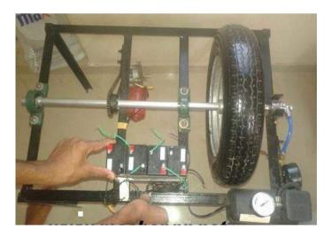
In this system, compressor is connected to wheel with the help of hoses through a rotary joint. Pressure sensor and control circuit are connected between wheel and compressor. Two limits (upper limit and lower limit i.e. 20psi and 30 psi respectively) are set in the control circuit for automatic start and stop of compressor. Compressor works on 12V DC supply that is either a car battery or bike or an adapter.
