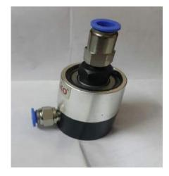
Rotary joint or a Rotary Union is a device that provides a seal between a stationary passage and a rotating part. Stationary passage may be a pipe or tubing; whereas rotating part can be a drum, spindle or a cylinder. Thus it permits the flow of the fluid into and/or out of the rotating part. Generally the fluids that are used with the rotary joints and rotating unions are steam, water, thermal oil, hydraulic fluids etc.
