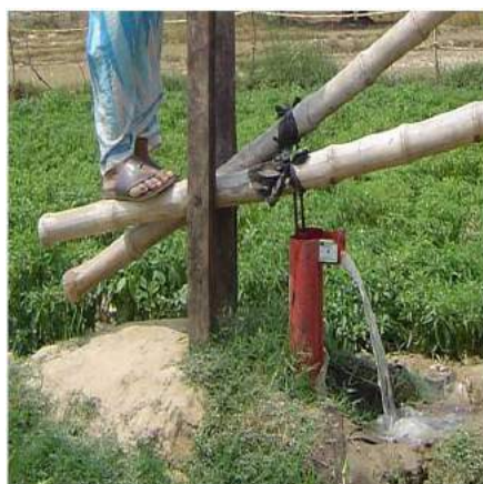
Fig.1. An example of a class I lever in the Bangladesh treadle pump
