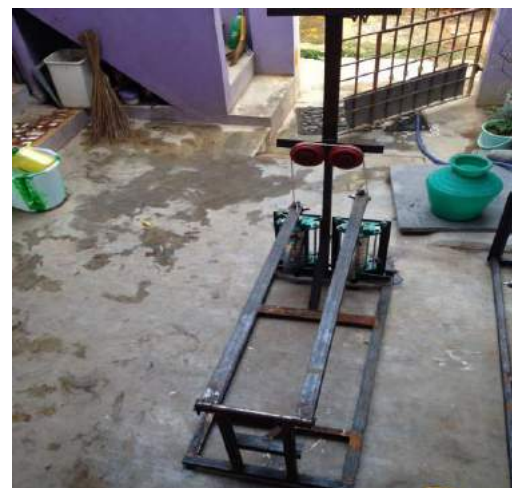
Fig.8.FABRICATION OF TREADLE PUMP
