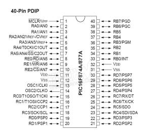
They are typically designed using CMOS (complementary metal oxide semiconductor) technology, an efficient fabrication technique that uses less power and is more immune to power spikes than other techniques.
