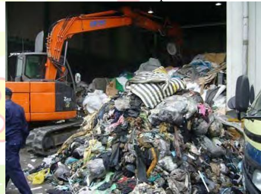
Figure 3.4 Heavy duty machine to feed wastes (150 kg/h capacity)
