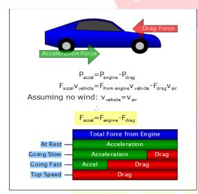
The engine exerts a force, while the aerodynamic drag opposes the engine's force. The remaining force from the engine is used for acceleration.
