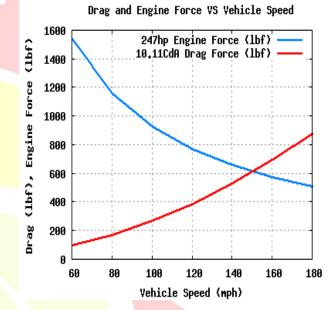
The above graph shows the force that the engine can exert, and the force due to aerodynamic drag. When the drag force becomes equal to the force the engine can exert, the car reaches its drag-limited top speed. In this case, the car's top speed is approximately 150mph.
