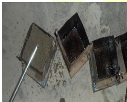
Figure – Casting of Mortar Cubes
