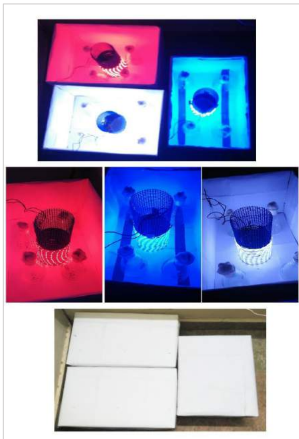
Fig 9. Closed LED light set-up for efficient algal growth
