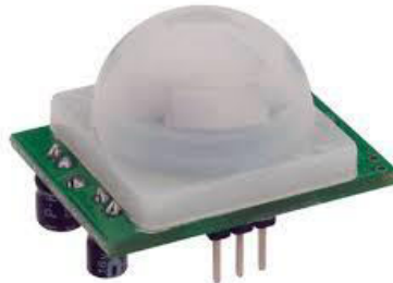
Fig4.3 Passive Infrared Sensor for Animal Capture
