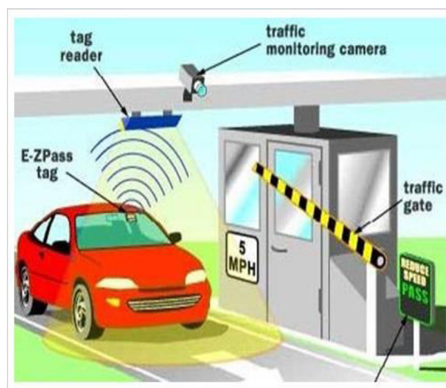
Fig: 2.4. Passive RFID toll collection system
