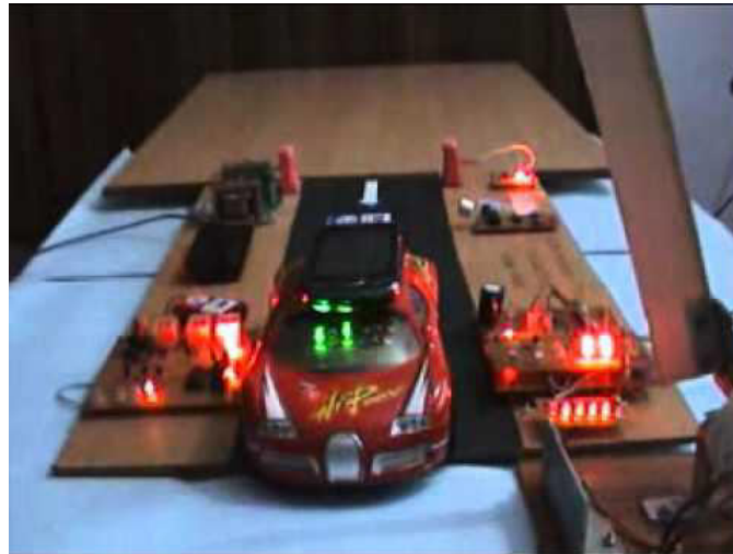
Fig: 5.1. Experimental implementation of electrical toll collection system
