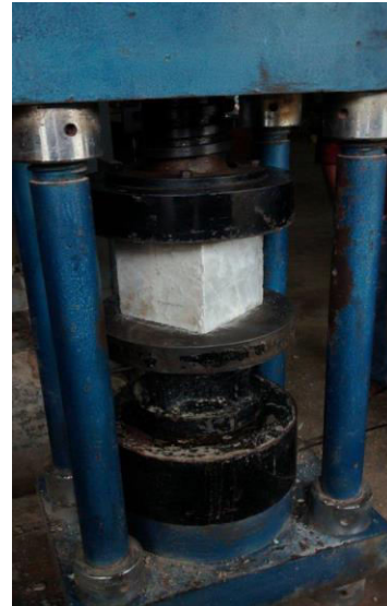
Testing of cubes for compressive strength
