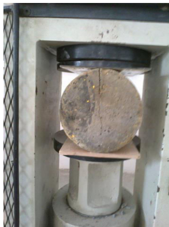
Fig split tensile strength on cylinder specimen
