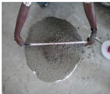
Fig Slump flow test for SCC
