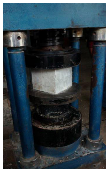
Testing of cubes for compressive strength
