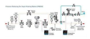
Schematic diagram for pressure reduced desuperheating station in thermal power station the stream control is using the integrated circuit (I.C). By this method we are overcoming the disadvantage of old technology used in the thermal power plant. This new method greatly reduces the huge reduction of human interaction with the thermal boiler. This is mainly used to control the pressure and temperature of steam for heating the boiler. Mainly reduce the wastage.
