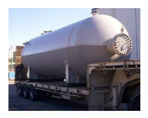
The development of Dewar vessel represents such an improvement in cryogenic fluid storage vessels that it could be classed as a "break-through" in container design. The high performance storage vessels in use today are based on the concept of the Dewar design principle a double walled the space between the two vessels filled with an insulation and container with the evacuated from the space. Improvements have been made in the insulation used between the two walls.
