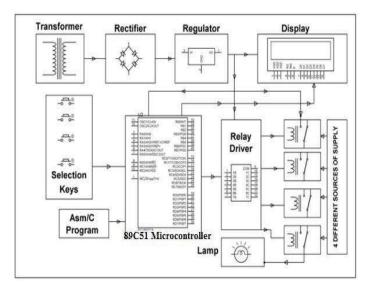
Fig.1 Block diagram of overall proposed system
