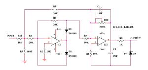
Current sensing circuit consists current transformer, shunt resistor, full waveprecision rectifier and finally a filter. The secondary of the current transformer should not be left open if there is any current in the primary, the entire primary voltage become the induced voltage for the secondary. Operation is same as that of voltage sensing circuit except a shunt resistance is used to convert current to voltage
