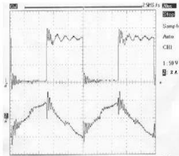
Fig. 9. PWM signals before and after optocouplers
