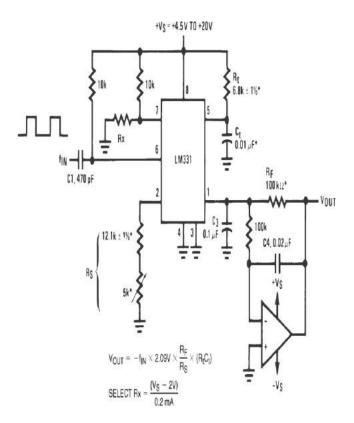
In this circuit, a pulse input at fin is differentiated by a C-R network and the negative-going edge at pin 6 causes the input comparator to trigger the timer circuit. Just as with a V-to-F converter, the average current
