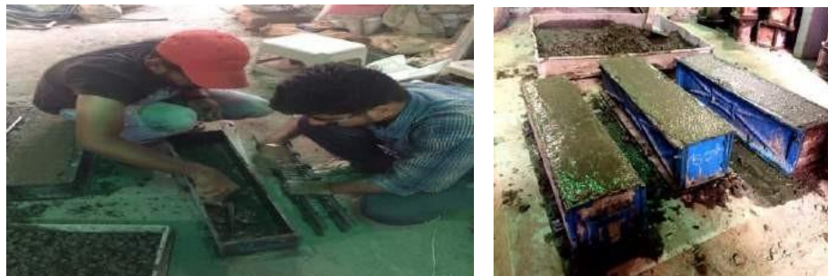
Fig. 2 Casting of Beam Molds
