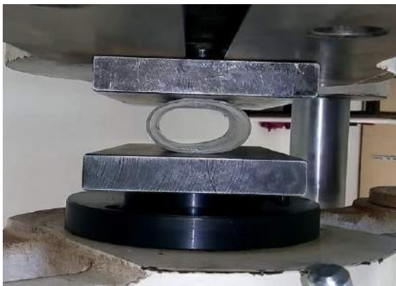
Fig. 6. Failure of specimens under lateral crushing loading at a rate of 1 mm/min
