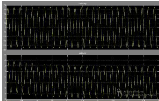
Fig.5. Output of load voltage and load current
