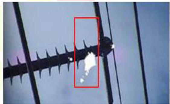
Fig. 5. Corona discharge on Polymeric Outdoor Insulators
