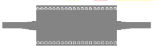
Fig.4 Structure of the SIW with Microstrip tapered transitions
