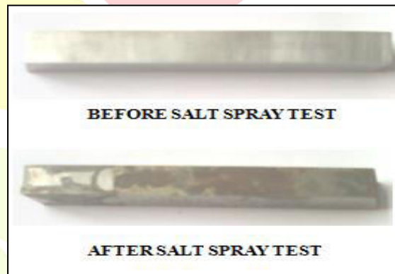
Fig.7. Photograph of the shallow Cryogenic treated specimen before and after the Salt spray test
