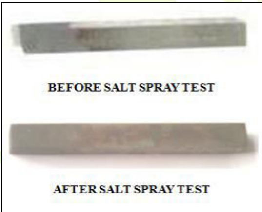
Fig .6. Photograph of the Tungsten carbide coated specimen before and after the Salt spray test
