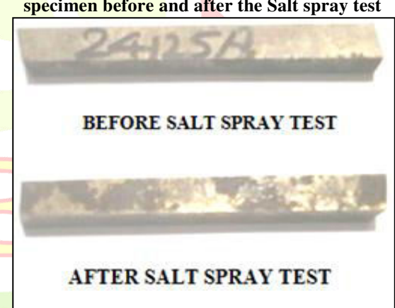
Fig .8. Photograph of the deep Cryogenic treated specimen before and after the Salt spray test
