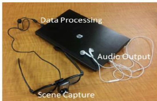
Fig. 3. Snapshot of our demo system, including three functional components for scene capture, data processing, and audio output.
