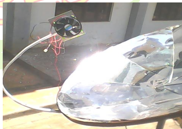
Figure 2. Parabolic Collector with Forced Air Circulation
