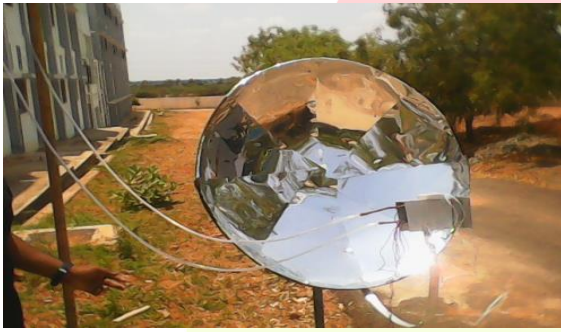
Figure 3. Parabolic Collector with Natural Convection
