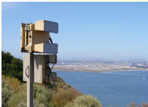
Fig 1.3.1- Blighter coastal security radar (Point Loma, San Diego, CA, USA)
