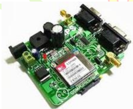
Figure 4 sim908 GSM/GPS module
