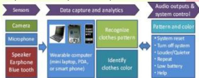
Fig. 2. Overview and architecture design of the camera-based clothing pattern recognition system for blind and visually impaired persons.
