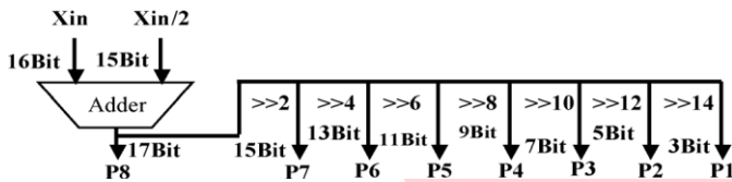
Fig -2: (Module 1) Partial product generator.
