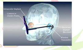
When received in the implanted chip, the digital information is transformed into electrical impulses sent into the ganglion cells. From there, the brain takes over as the information travels down the optic nerve to the visual cortex at the back of the brain. The whole process occurs extremely rapidly, so that patients see in real-time. This is important any noticeable lag could stimulate the "vestibularocular reflex", making people feel dizzy and sick.
