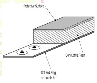
If the resistance measurement is taken between opposing surfaces of the elastomer, the upper contacts have to be made using a flexible printed circuit to allow movement under the applied force. Measurement from one side can easily be achieved
