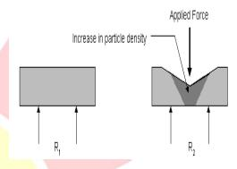
The basic principle of this type of sensor is the measurement of the resistance of a conductive elastomer or foam between two points. The majority of the sensors use an elastomer that consists of a carbon doped rubber. In the above sensor the resistance of the elastomer changes with the application of force, resulting from the deformation of the elastomer altering the particle density.
